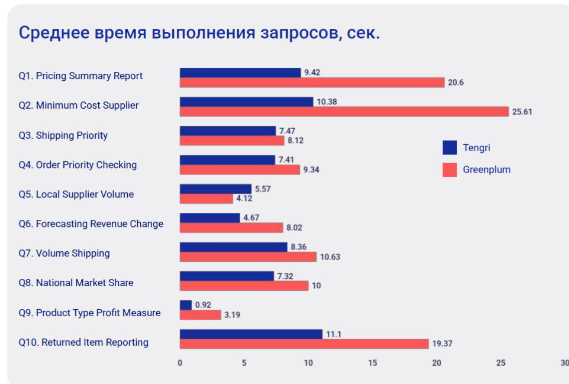
When the system is used by 10 analysts, Tengri outperforms **Greenplum** due to efficient resource utilisation without competition:
